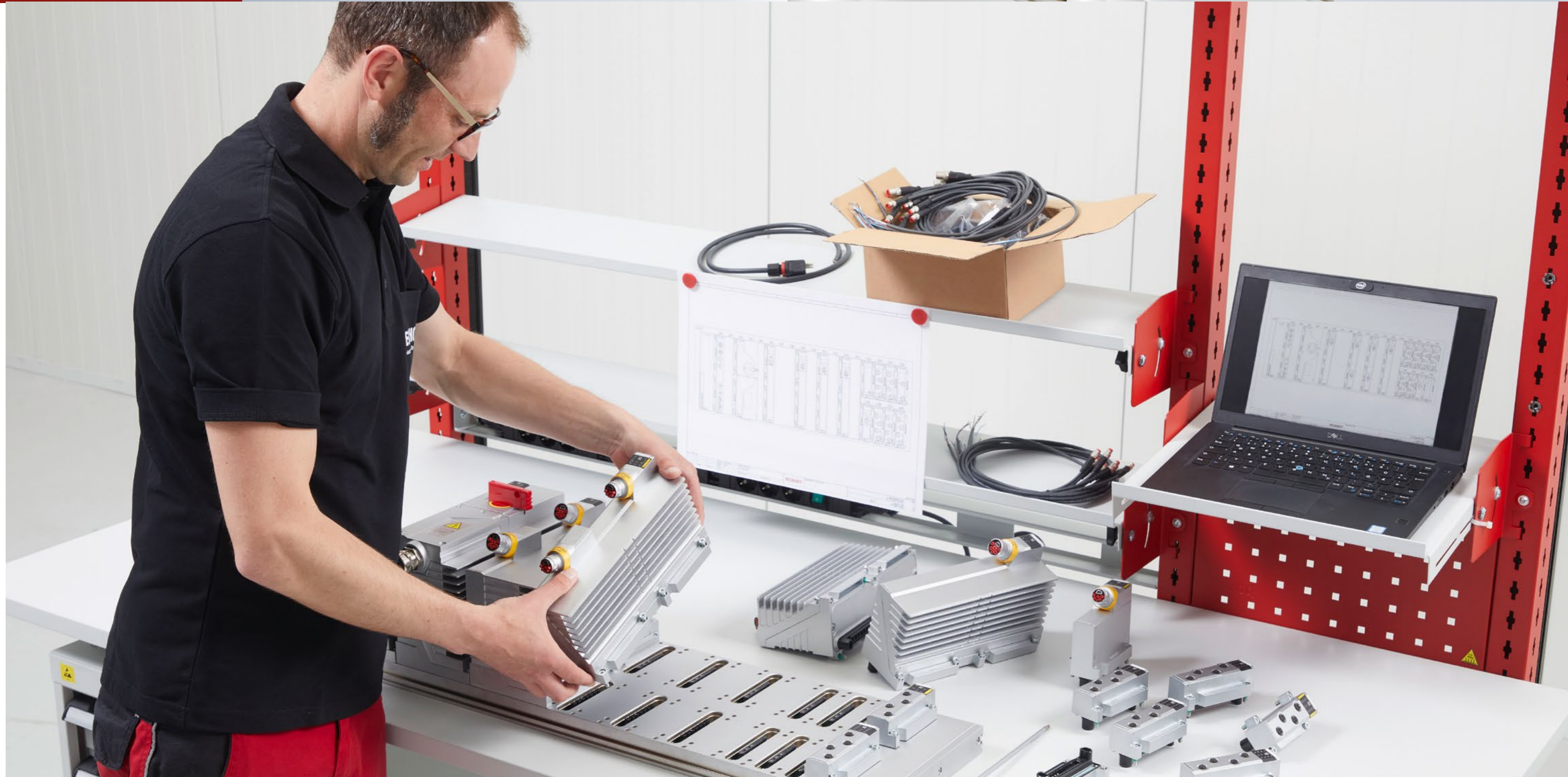
Step 1: Plug module according to mounting plan
