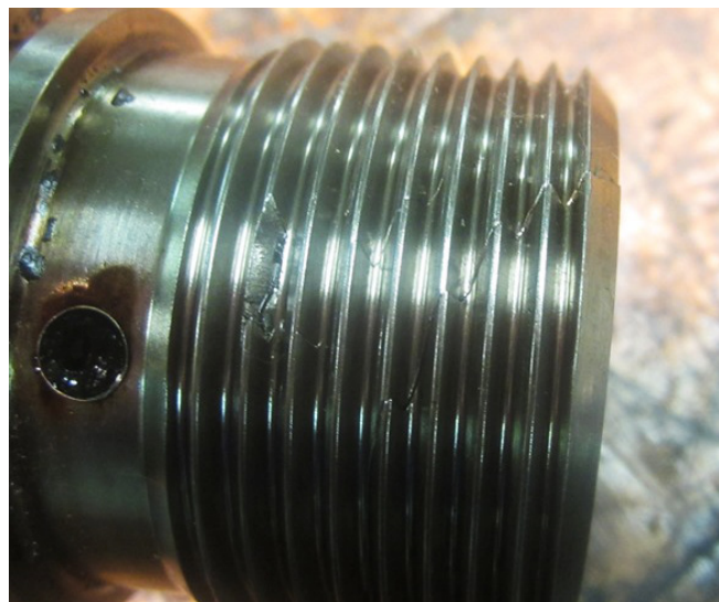
Cracked fuel oil pipe nipple
