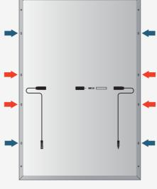
7.4 Installation precaution and instruction PV modules can be mounted to the substructure using specially designed module clamps.
