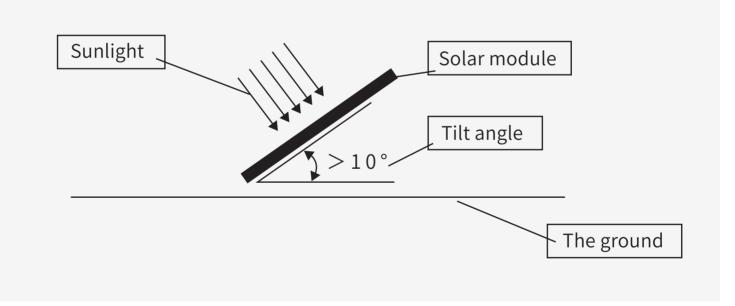
For installations in the northern hemisphere, it is recommended that modules should preferably face south, and for installations in the southern hemisphere, it is recommended that modules should preferably face north. If solar modules are mounted at a different elevation and azimuth angles, the annual energy production may potentially be adversely impacted.
