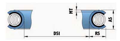
Seal: DSI = DG + DC + (Plating thickness X 2) Groove: DG = DSI - DC - (Plating thickness X 2)
